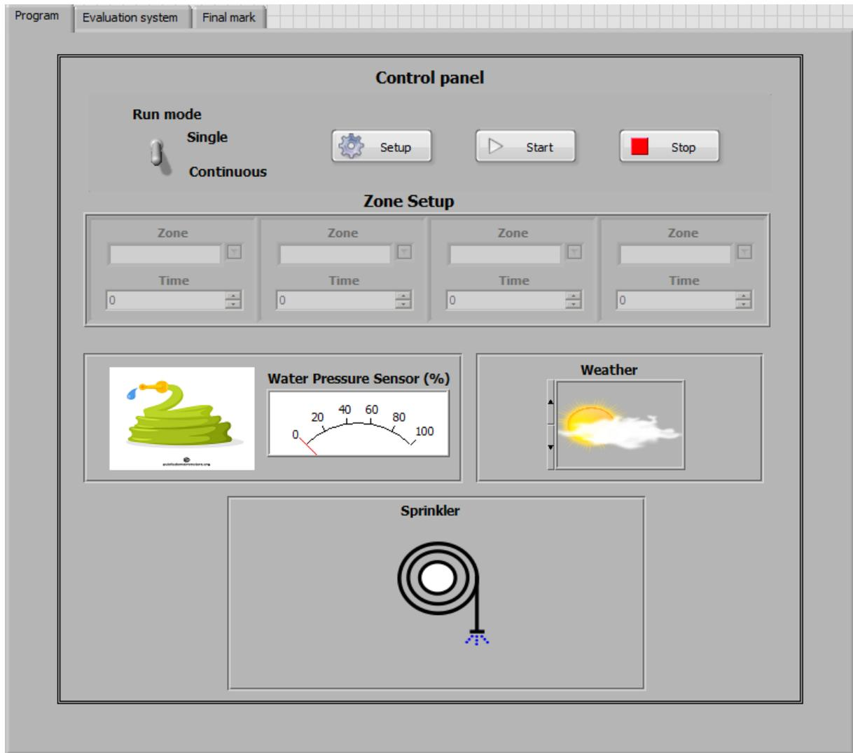
Figure 1: *Front panel* of a sprinkler simulator.
